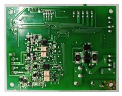
WS-DALI2-4C-TU Rated Input Voltage 12VDC Output Specifications 4ch/Remote control Relay
