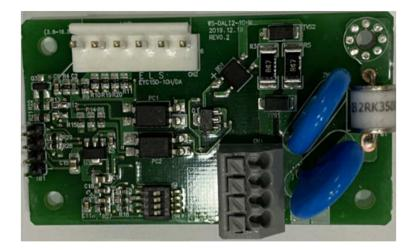
WS-DALI2-1C-M Rated Input Voltage 6.3~16.5VDC Output Specifications 4ch/0~100% 1kHz PWM
